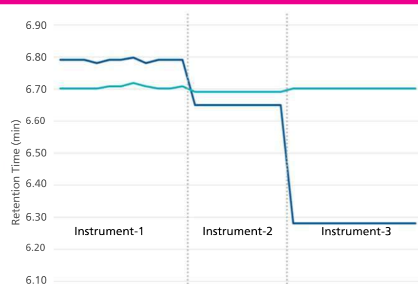
Figure 1: One month of daily retention times are shown for three instruments using RTL (teal) and without RTL (blue).
